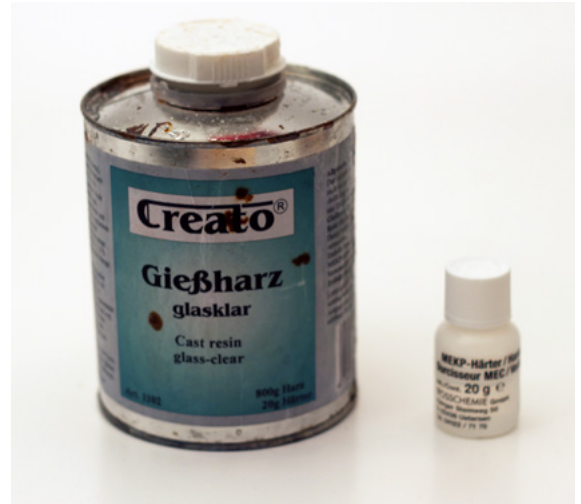
Cast resin comes in many shapes and colours. Often, it is bought in cans like this with a tiny bottle of hardener.
