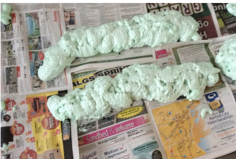
Expanding foam grows to about 20 times the size after it has been sprayed.
