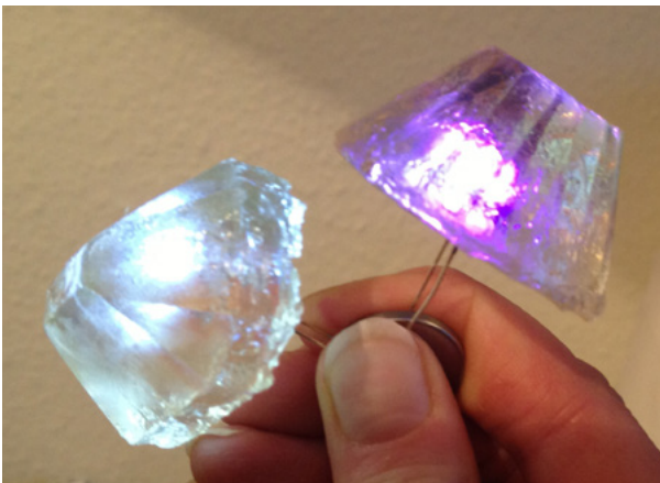
Resin gems cast in an ice cube tray with LEDs inside. Not yet sanded or lacquered.
